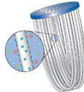
Diagram of a Hollow Fiber Membrane
